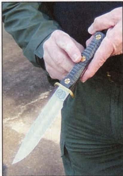
The X-head screws allow the handle scales to be removed for cleaning and other purposes. For maximum durability, Ahern chose grooved Micarta scales. Walnut is another option.
